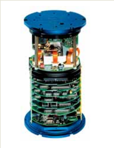
Figure 1 – Example of an application for motion sensors (MRU – Motion Reference Unit)
